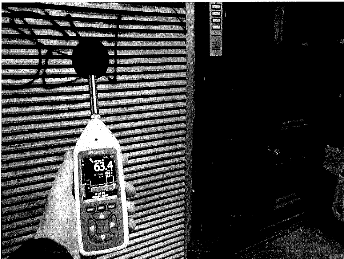
Figure 4: Plant noise at 1m.
